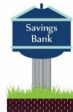
Example Concealed Pole Support Using Cladding
