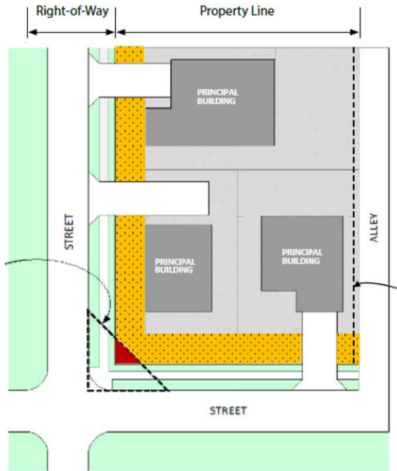
Figure 2.16.05(A): Residential Zoning Fence Requirements
